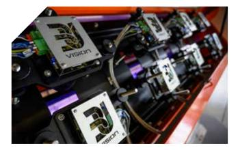
High resolution multispectral cameras SWIR (1024 pixel), up to 4 wavelengths. These cameras allow unreachable results until now, recognising polymers, selecting shells and foreign bodies in dried fruits and where there are chemical differences even if not visible by human eyes. Simultaneous use of RGB, SWIR and IR optical systems: up to 8 frequencies (the standard on the market for these sorters is usually not more than 4 frequencies).
