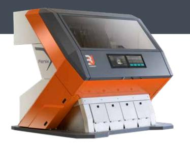
State of the art Ev, 3.2mm pitch: with custom design and specification, can reach top values in duration and speed, practically double the number of electrovalves in each chute. This to increase production speed, reducing the quantity of good products wrongly expelled (reject products more concentrated) and allowing to reduce air consumption.
